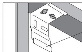
Make sure the release tab is always mounted on the bottom.
