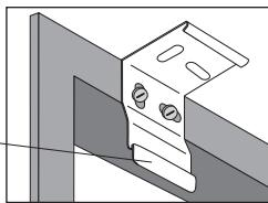
Make sure the release tab is always mounted on the bottom.
