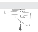
Low light gap wedges can be used to reduce the top light gap when the shade is mounted fully recessed . The wedge is placed between the mounting surface and the bracket with the tabs on the wedge facing down and the thick end of the wedge toward the back of the bracket.
