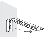
Position screw in center of slot so you can adjust position of bracket as necessary
